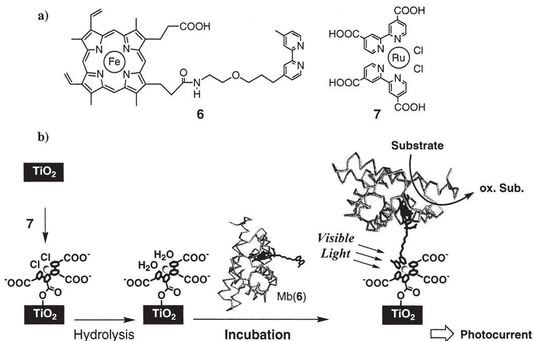
FIGURE 8 (a) Molecular structure of bpy-appended proporphyrin IX **6** and bis-Ru<sup>II</sup>(bca)<sub>2</sub>Cl<sub>2</sub> **7** (b) Immobilization scheme of Mb(**6**) on TiO<sub>2</sub>/ITO electrode via coordination chemistry.
