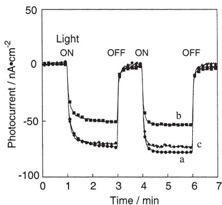
FIGURE 9 Photocurrent generation of Mb-Ru<sup>II</sup>(bpy)<sub>3</sub>-TiO<sub>2</sub>/ITO electrode in the presence of guaiacol as an oxidative substrate. (a) intact Mb-Ru<sup>II</sup>(bpy)<sub>3</sub>-TiO<sub>2</sub>/ITO electrode after incubation, (b) after treatment with 3M Gdn-HCl, (c) after re-incubation of apo-Mb with electrode of (b)
